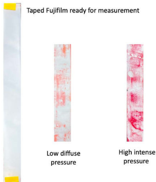
Figure 2. Shows how the FujiFilm correlates with the amount of pressure exerted on the film. Note how this film can detect not only intensity of colouration but also whether it is a dense or diffuse colouration.
